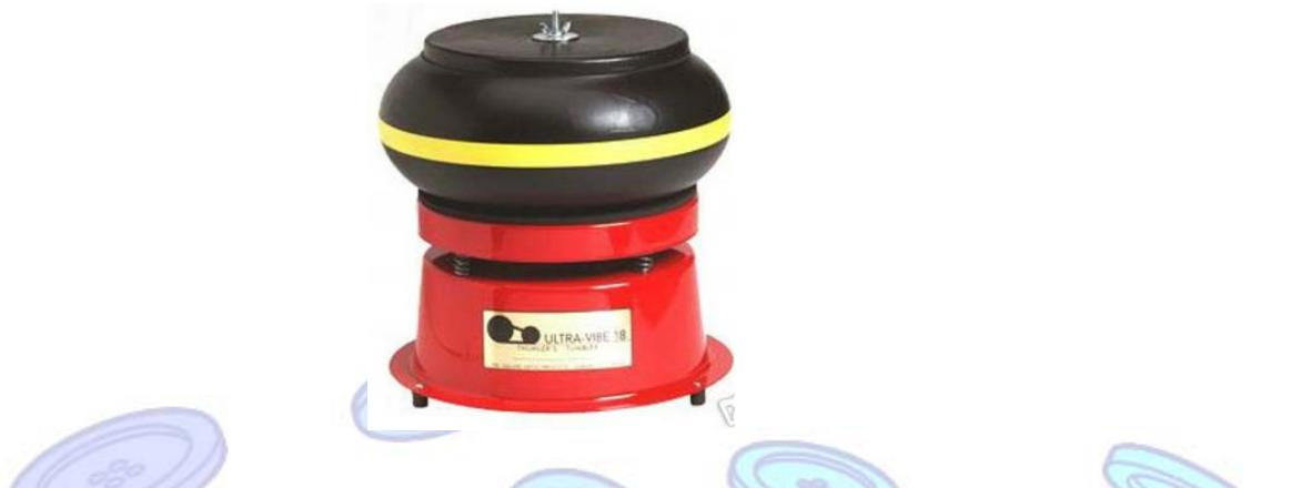
The buttons are vibrated in the machine, along with ground walnut hull media. (Ground corn cobs can also be used, but I have been told that they need to be replaced more frequently than the walnut shells.)
